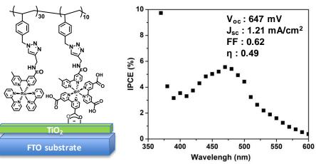
Immobilization of a Ru-polychromophore onto a mesoporous  $TiO_2$  film (left); Solar cell characteristics of Ru-polychromophore anchored  $TiO_2$  films (right).
