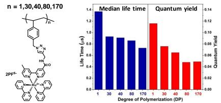
A series of Ru-polychromophores constructed with varying chain length and low polydispersity index (<1.4) (left) and photophysical studies as a function of polymer chain length (right).
