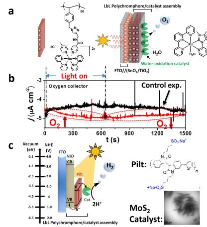
(a) Schematic illustration of light-driven water splitting processes in LbL/TiO $_2$  photoanode. (b) Current–time traces at an FTO collector electrode measured concurrently with the photoelectrochemical–time trace. (c) Energy diagram of light-driven water splitting processes in a photocathode.
