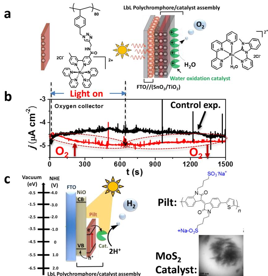
(a) Schematic illustration of light-driven water splitting processes in LbL/TiO<sub>2</sub> photoanode. (b) Current-time traces at an FTO collector electrode measured concurrently with the photoelectrochemical-time trace. (c) Energy diagram of light-driven water splitting processes in a photocathode.
