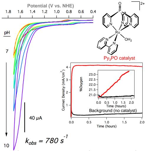
Conditions: 0.1 M phosphate in H<sub>2</sub>O, glassy carbon or ITO working electrode, Pt counter electrode
