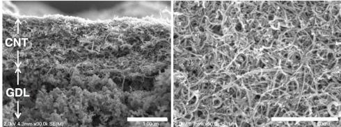
**Structure and Operation of GDE:** (Top) GDE immobilized with Ir pincer dihydride catalyst **1** for electrochemical reduction of  $CO_2$  to formate at the interface of  $CO_2$ /water.
